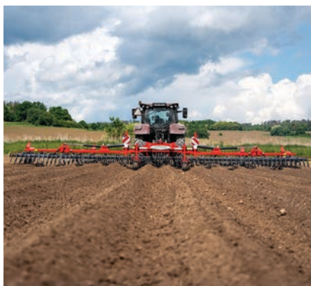
Pöttinger TINECARE provides a mechanical weeding process.
