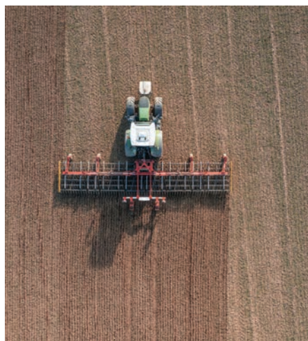
The interrow tines carefully pick up unwanted weeds or bury them in soil.
