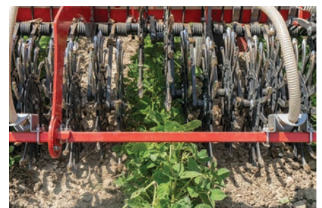
Pöttinger ROTOCARE comprises of rotary stars that carefully pick up soil.
